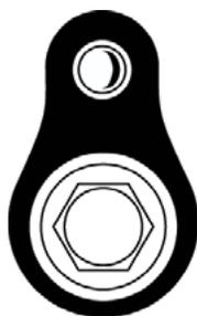
**Bypass** : Indicates whether the effect is engaged; a turquoise light indicates the effect is on, while a red light indicates the effect is bypassed. The light will turn blue when recording knob movements.
